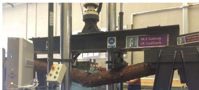
Figure 1: Four point bending test setup
