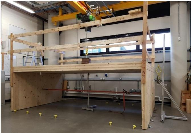
Figure 4. Static point load deflection measurement, one-way long span platform construction at NUI Galway
