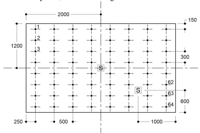
Figure 5. Transducer locations: 500 x 300 mm grid of 64 measurement points. Two alternative shaker locations, midspan and quarter-span
