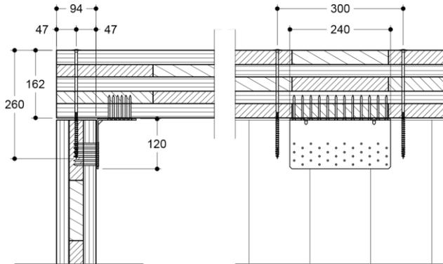
Figure 2. Assembly F, partially threaded vertical screws at 300 mm c/c with 240 x 93 x 120 mm brackets at 800 mm c/c
