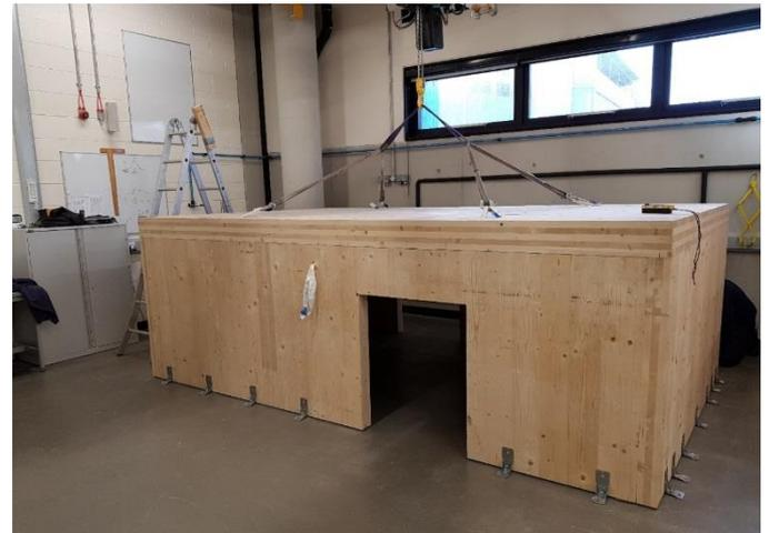
Figure 3. Assembly P, erection of two-way span platform construction at NUI Galway
