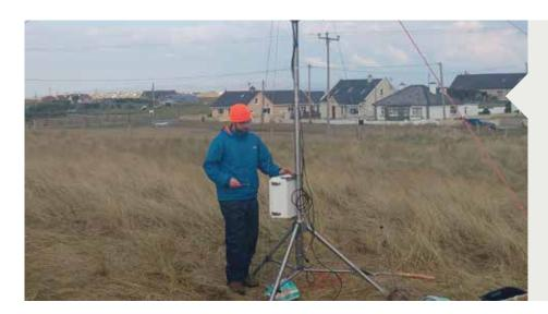
Geography PhD student Guillermo Castro Camba is pictured setting up a portable Automatic Weather Station on the sand dunes in Magharees (An Machaire), Co. Kerry. He is using the low-power device to collect high frequency meteorological measurements in order to examine how the weather impacts our coastline. The research is part of an OPW-funded project by Dr Eugene Farrell and Dr Kevin Lynch (Geography) that examines long-term beach-dune response and recovery to storms.
