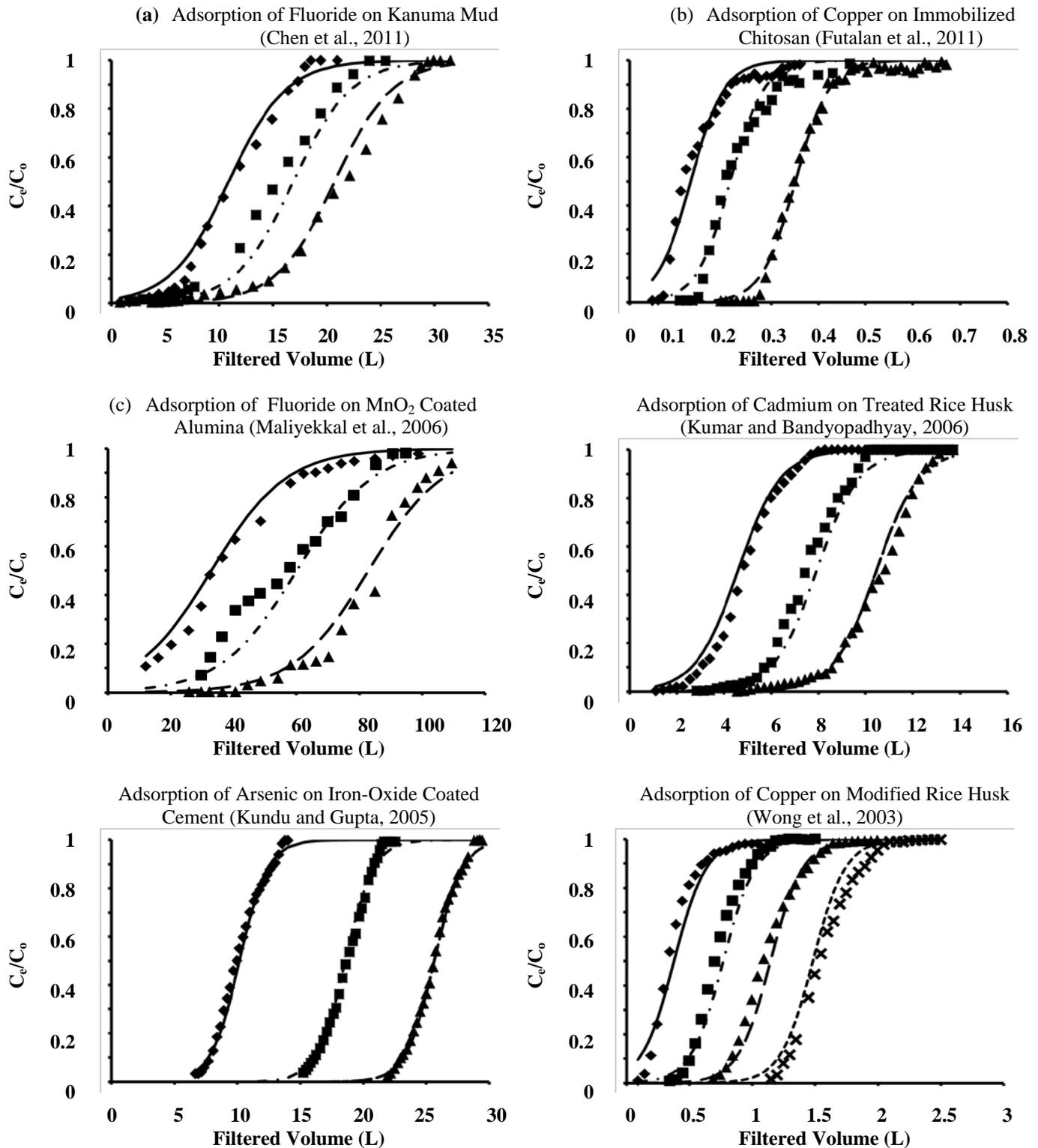
**Figure 5.5** Equation 10 fit to independent data sets of normalised pore/effluent contaminant concentration (y-axis) vs. filter loading/operating time (x-axis).
