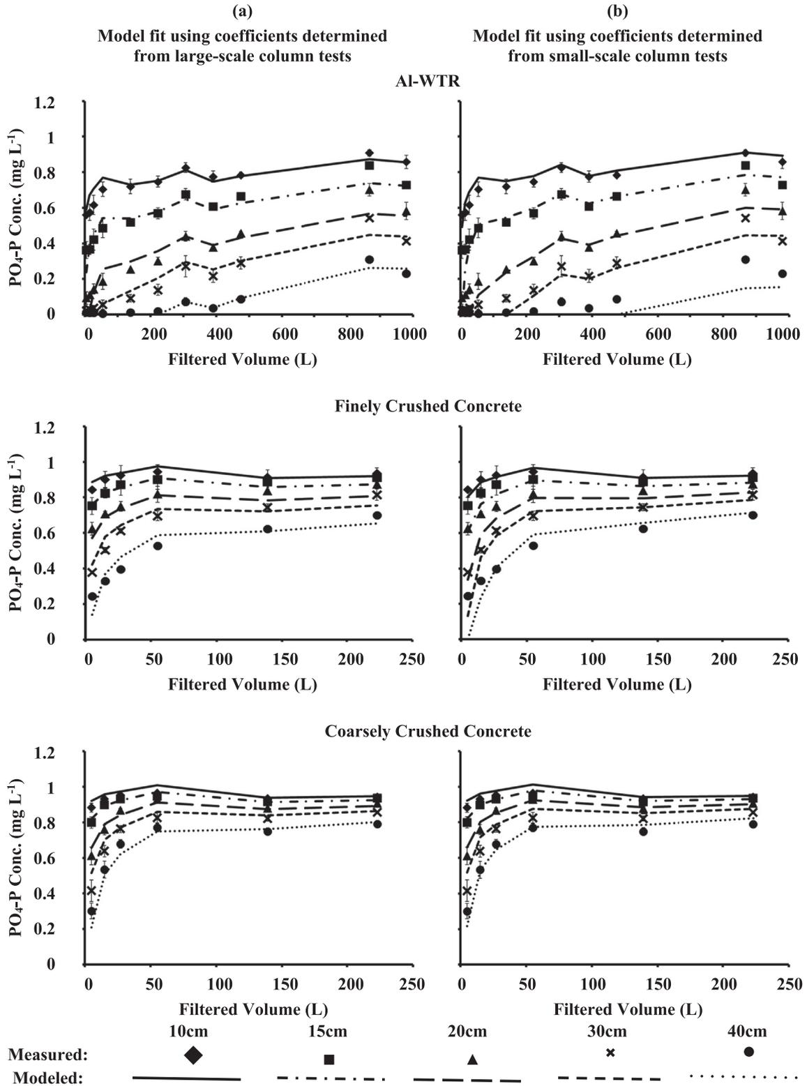
Fig. 3. PO<sub>4</sub>-P concentration (y-axis) vs. filter loading (x-axis) for large scale filter columns, showing (a) Eqn (16) fit directly to large scale column data, and (b) predictions made by Eqn (16) with model coefficients determined from small-scale column tests.
