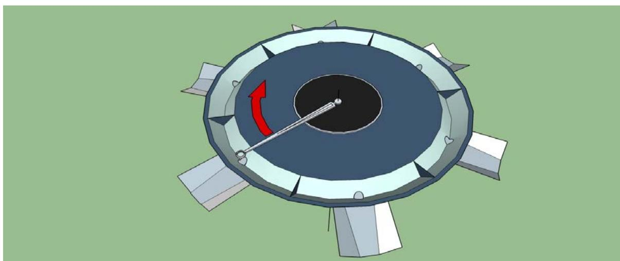
**Figure 2.3 Schematic of autosampler**
