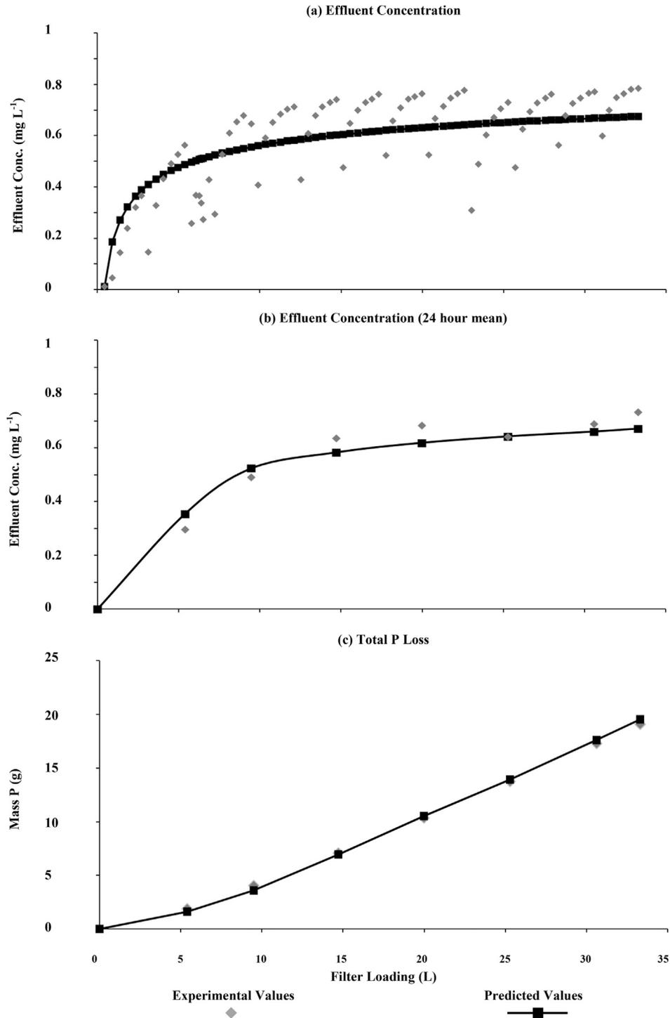
**Fig. 2.** (a) Comparison of predicted and observed progressions of effluent concentration (y-axis) vs. cumulative filter loading (x-axis), with predictions and observations made on a bi-hourly basis. (b) Comparison of predicted and observed daily mean effluent concentrations (y-axis) vs. cumulative filter loading (x-axis). (c) Comparison of predicted and observed cumulative P loss in effluent (y-axis) vs. cumulative filter loading (x-axis).
