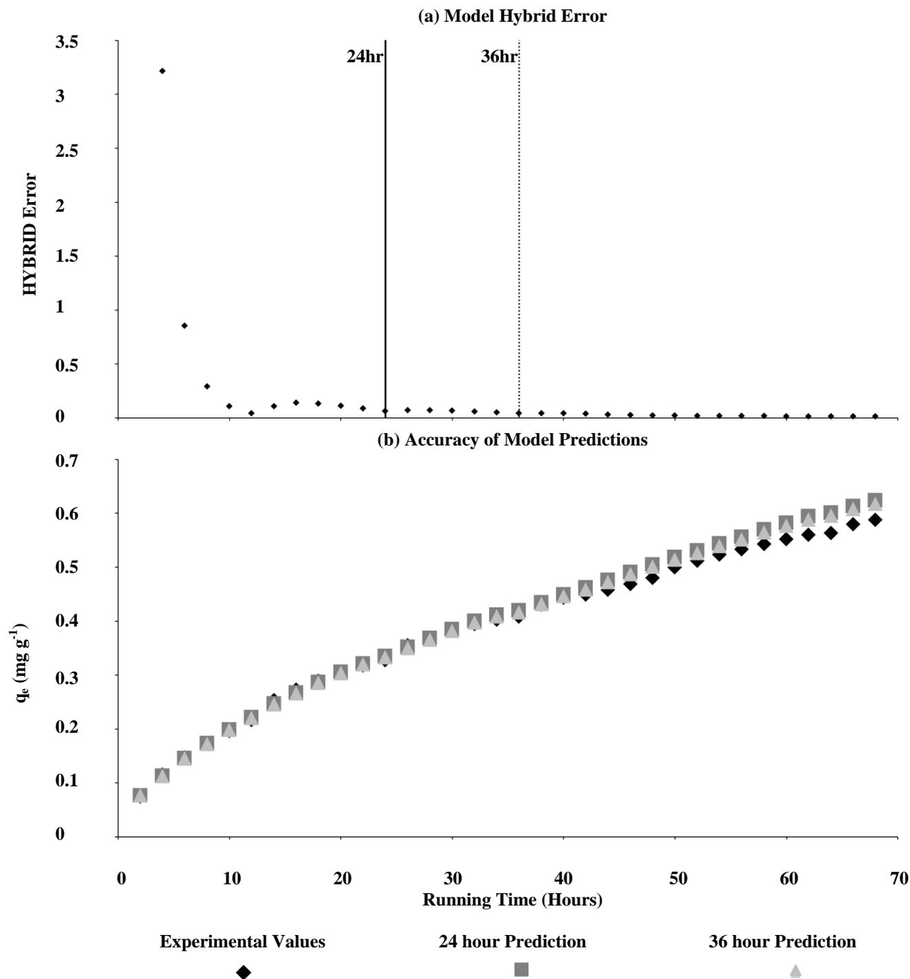
**Figure S4.2 (a)** HYBRID errors (y-axis) of models predicting 68 hours of adsorption column performance, against the time at which model predictions were made (x-axis). Model predictions were revised at two hour increments using increasingly more data as it was obtained.
