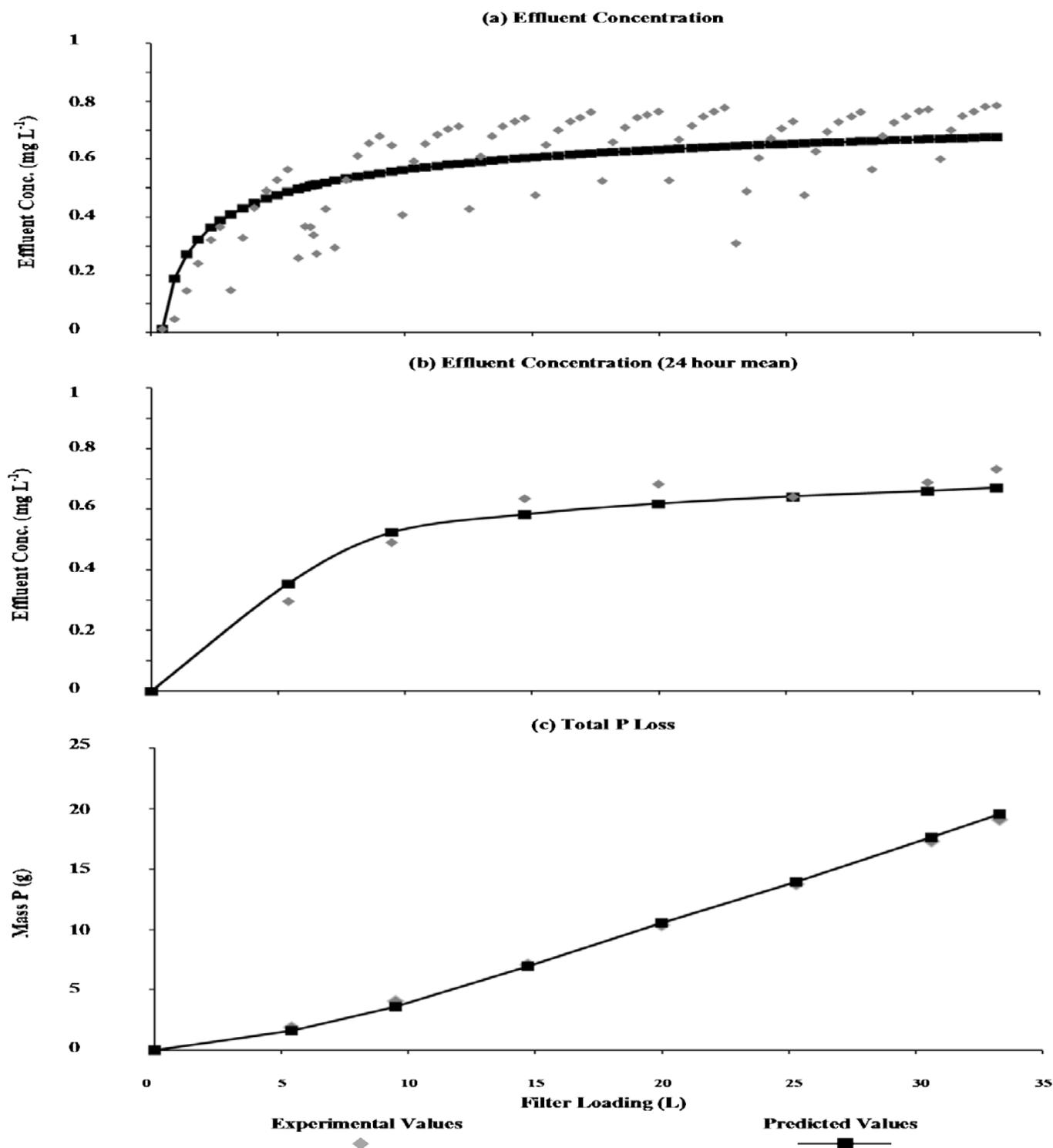
**Figure 4.2 (a)** Comparison of predicted and observed progressions of effluent concentration (y-axis) vs. cumulative filter loading (x-axis), with predictions and observations made on a bi-hourly basis.
