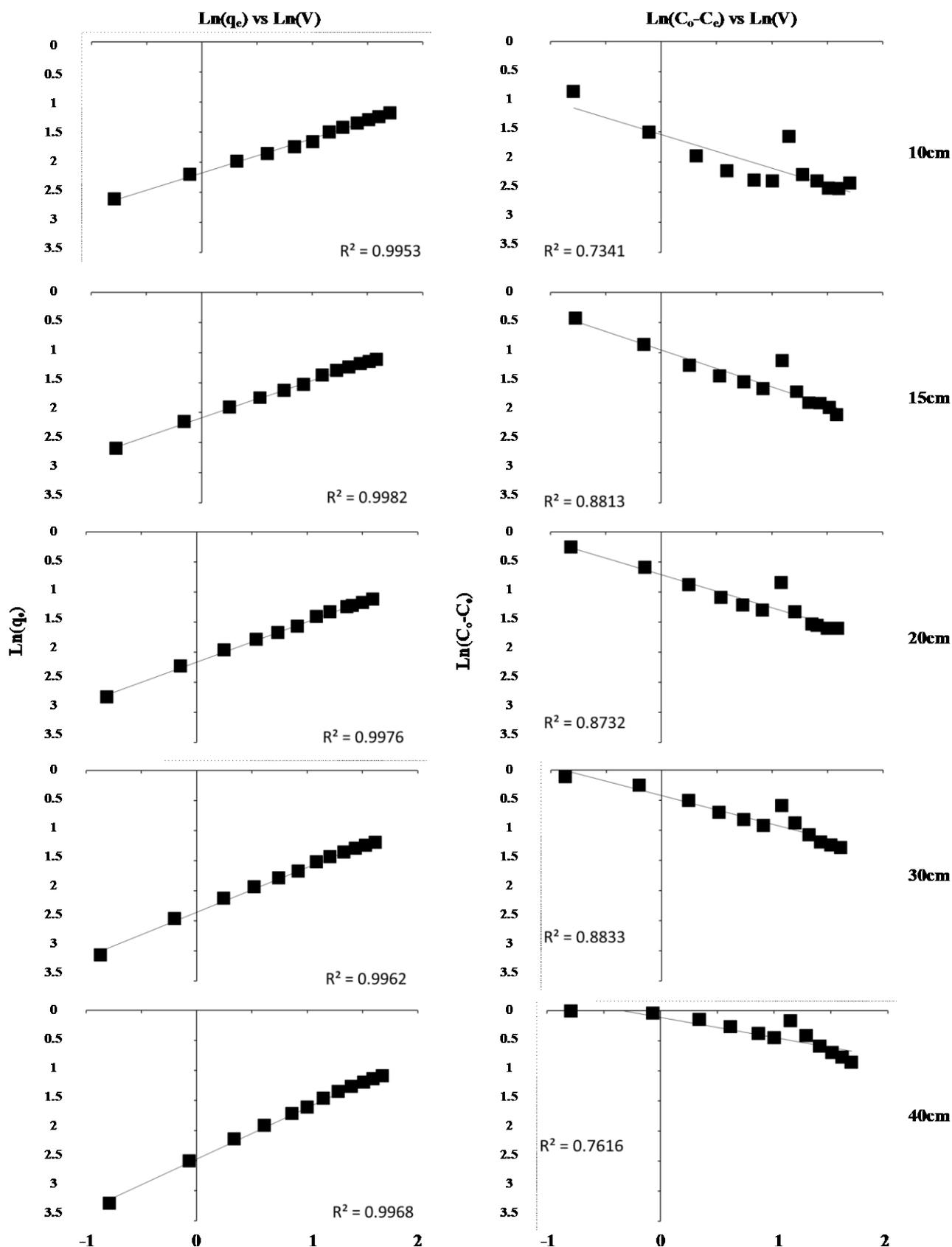
**Figure 4.5** Comparison of the linearity of plots of  $\ln(q_e)$  (left y-axis) vs.  $\ln(V)$  (x-axis), and  $\ln(C_0 - C_e)$  (right y-axis) vs.  $\ln(V)$  (x-axis). These plots are used to determine model coefficients by analysis of filter saturation or filter effluent concentration respectively.
