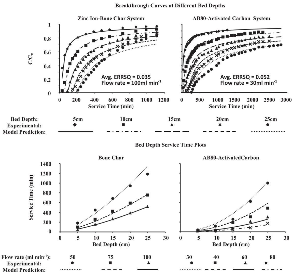
**Fig. 6.** (a) Eqn (16) fit to an independent data set of normalised effluent contaminant concentration (y-axis) vs. filter operating time (x-axis) for various filter-bed depths, and (b) plots of filter service-time (y-axis) vs. filter-bed depth (x-axis) compared to predictions made by Eqn (17) using the same model coefficients.
