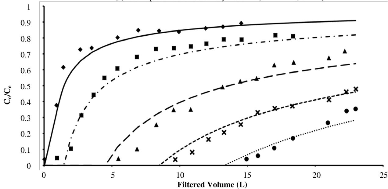
(b) Adsorption of Phosphate on Zirconium Loaded Okara (Nguyen et al., 2015)
