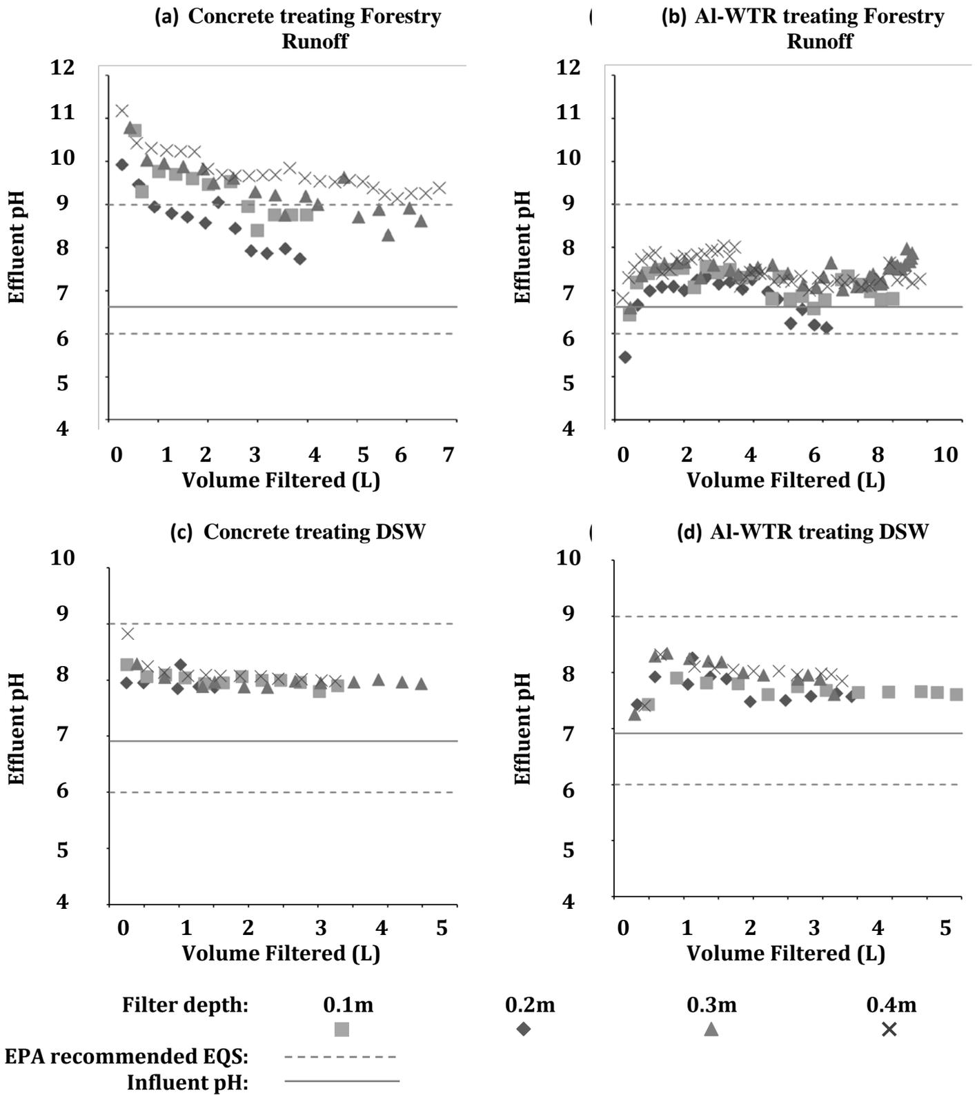
**Figure 6.3** Filter column influent and effluent pH and their relationship to EPA recommended environmental quality standards (EPA 2001).
