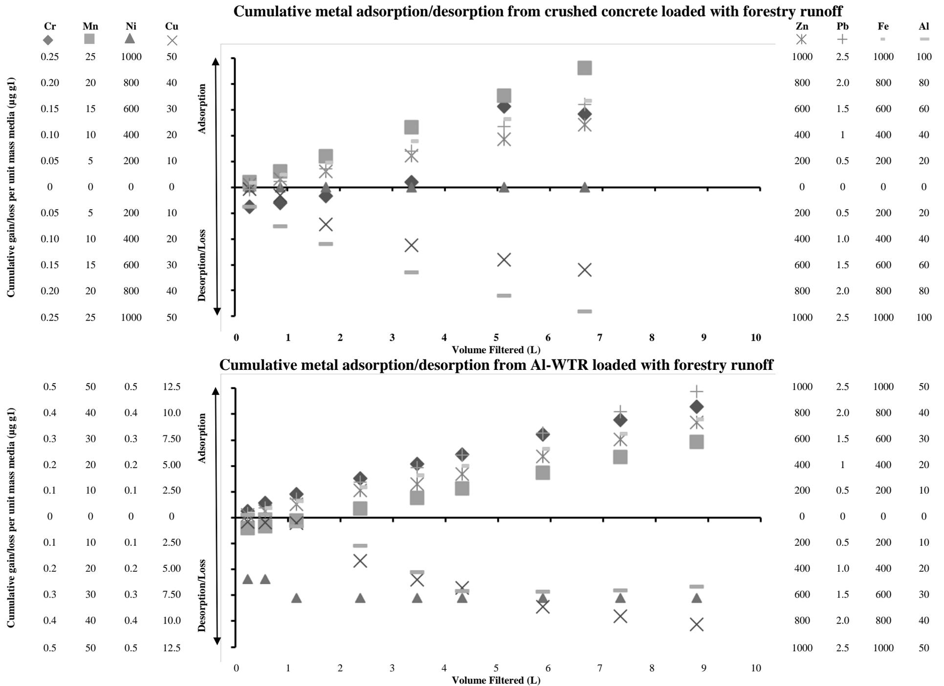
Figure 6.2 (a) Cumulative metal release/uptake by 0.4 m filter columns.
