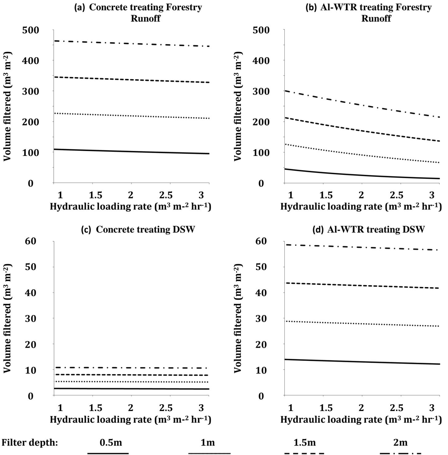
**Figure 6.4** Indicative full-scale filter lifespan to effluent breakthrough concentration of 10% filter influent concentration for filter-beds of various depths subject to HLRs of 1-3  $\text{m} \text{hr}^{-1}$ .
