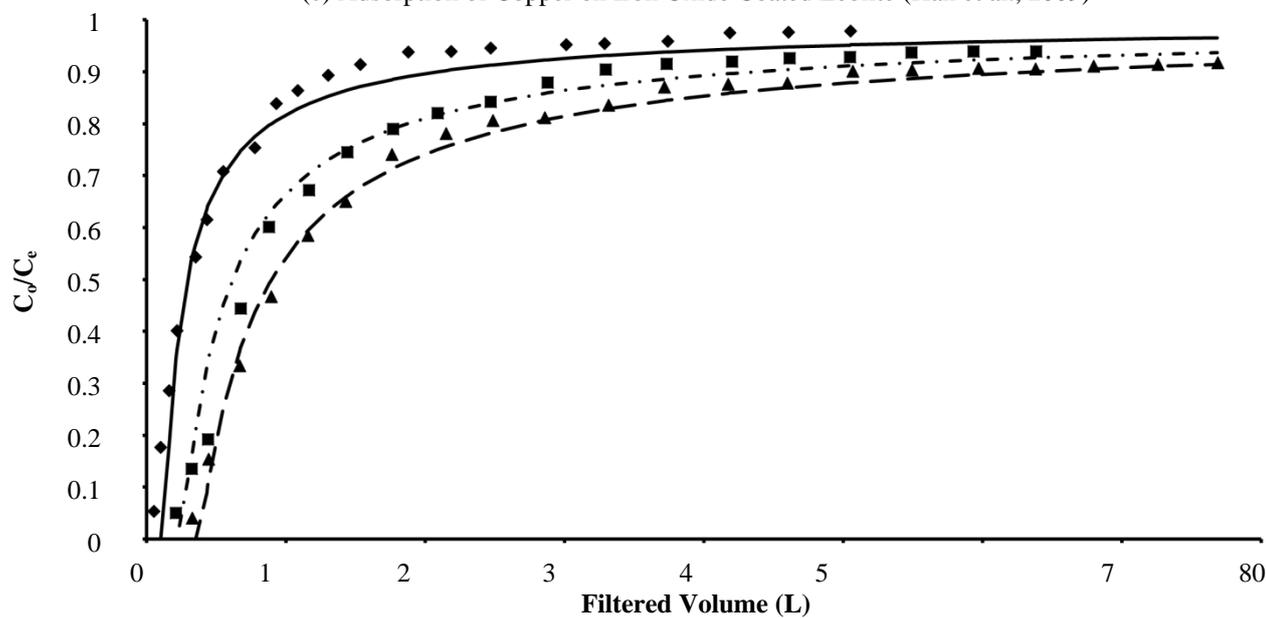
**Figure 5.4** Equation 16 fit to independent data sets of normalised pore/effluent contaminant concentration (y-axis) vs. filter loading/operating time (x-axis).
