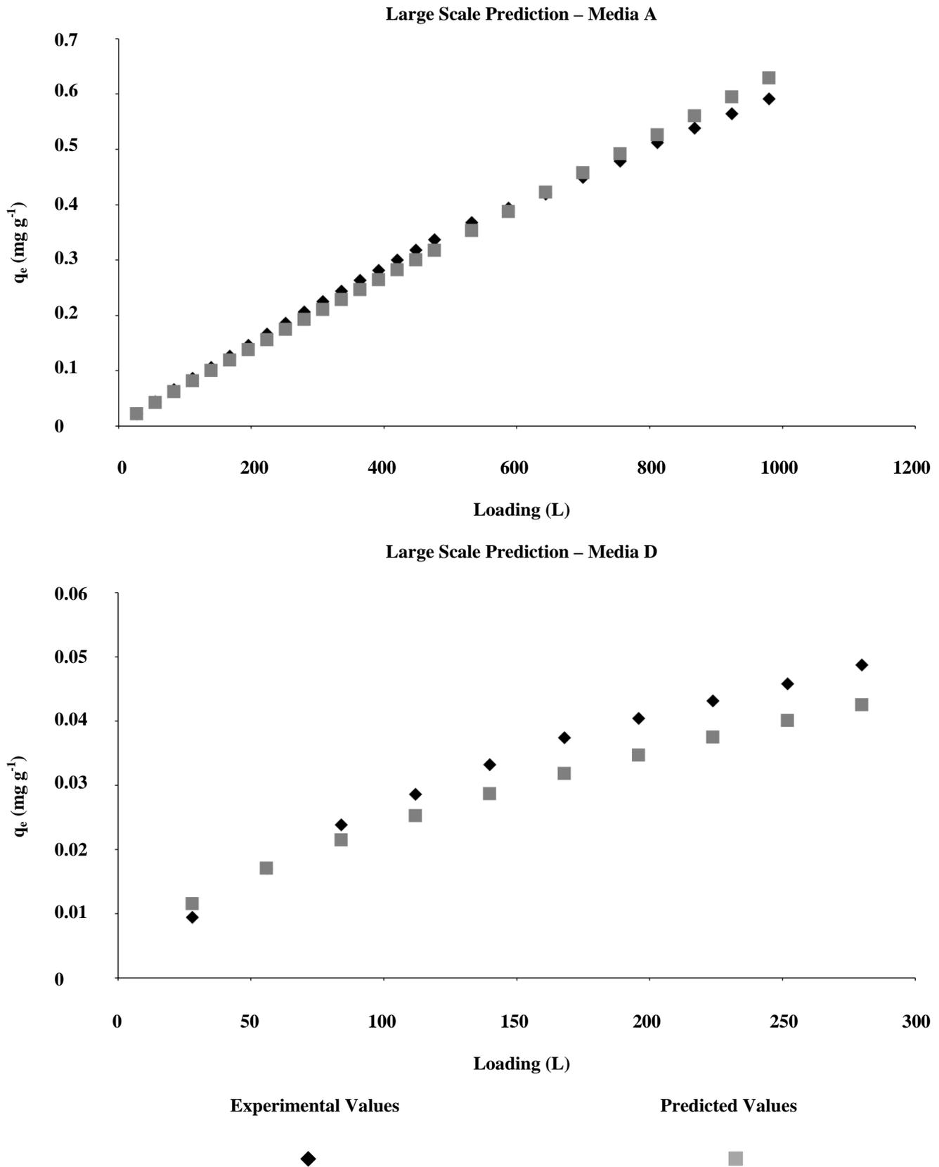
**Figure 4.3** Comparison of predicted and observed  $q_e$  values (y-axis) vs. filter loading (x-axis), demonstrating the ability of the proposed model to predict large-scale filter performance.
