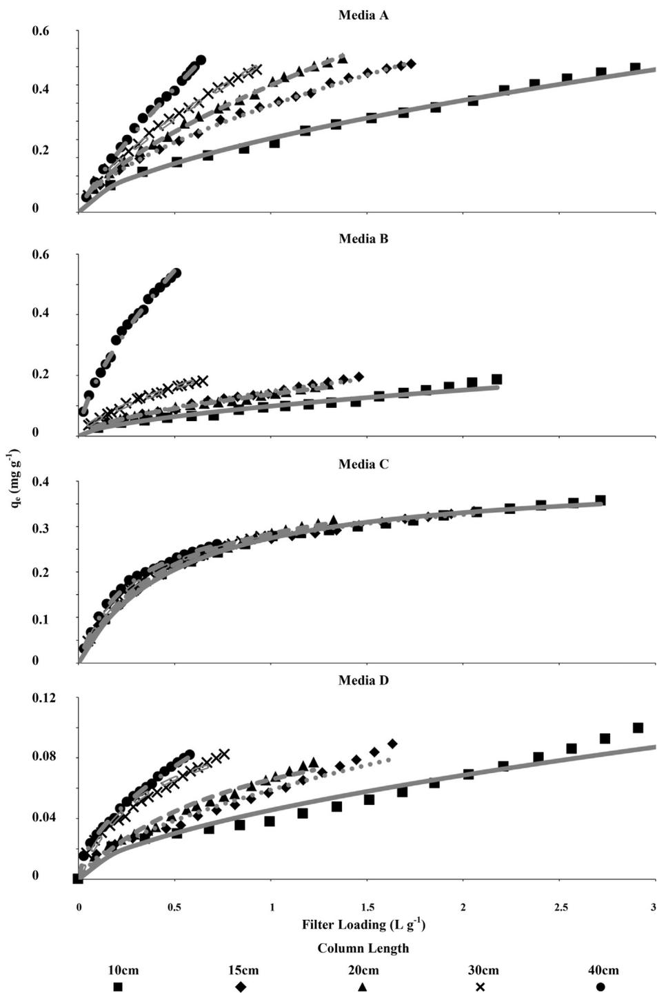
Fig. 1. Filter media P adsorption (y-axis) vs. filter loading (x-axis), showing observed progressions of media saturation and the goodness of model fit for each media and column length.
