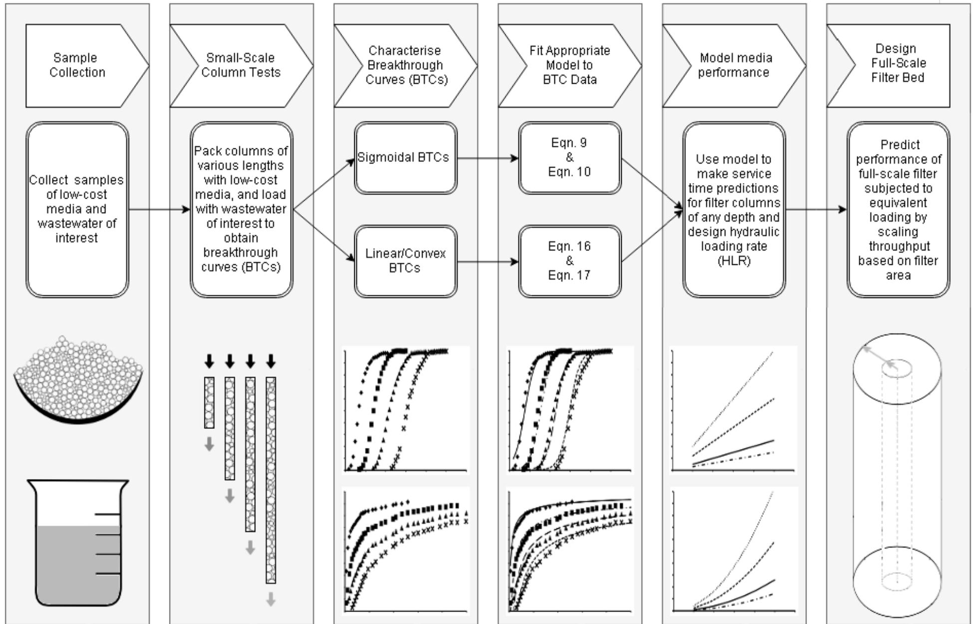
**Figure 5.1** Step-by-step schematic of the data collection and modelling procedure employed in this study.
