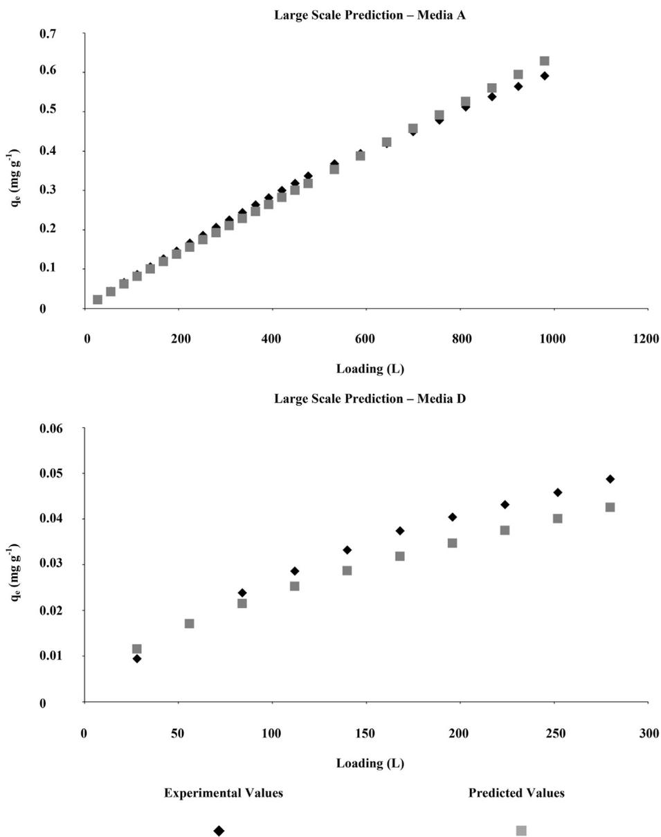
Fig. 3. Comparison of predicted and observed  $q_e$  values (y-axis) vs. filter loading (x-axis), demonstrating the ability of the proposed model to predict large-scale filter performance.
