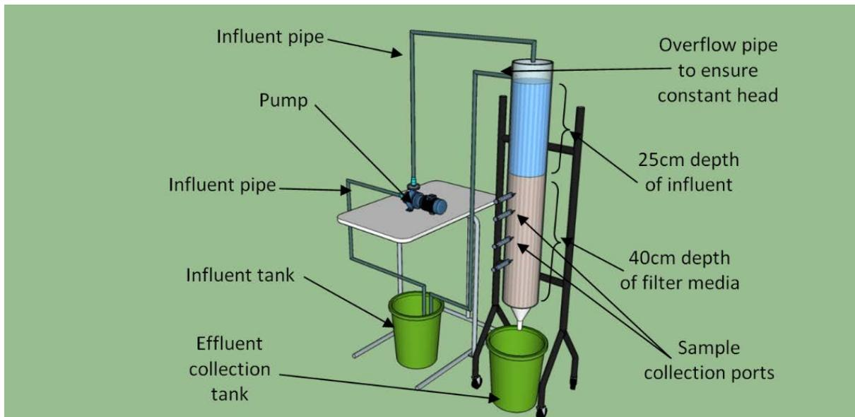
**Figure 2.1 Schematic of large-scale filter column experiment**
