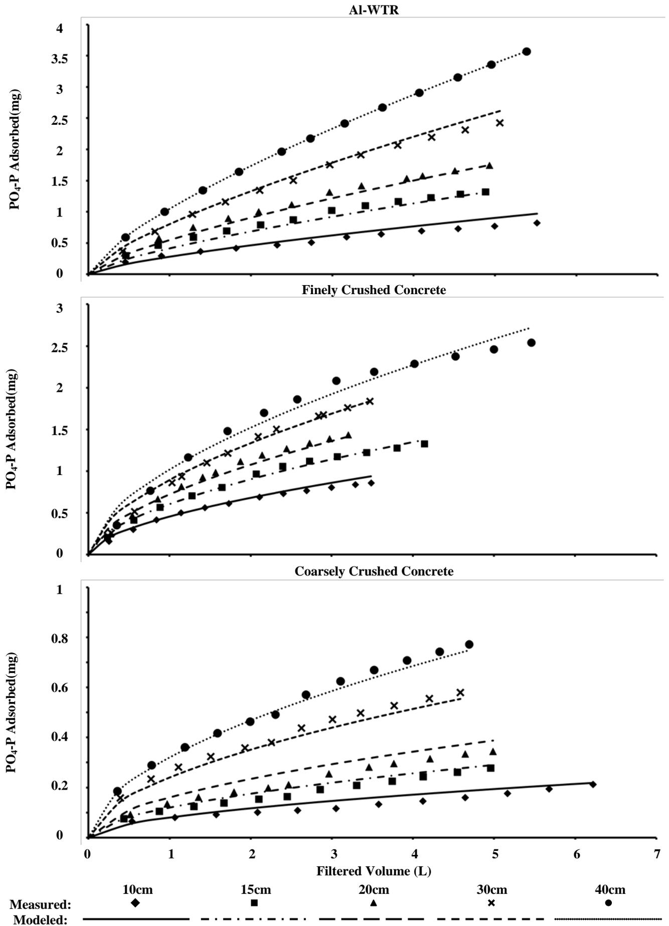
**Figure 5.2** Phosphorus retained by filter media (y-axis) vs. filter loading (x-axis) for small scale filter columns of various lengths and predictions made by Equation 15.
