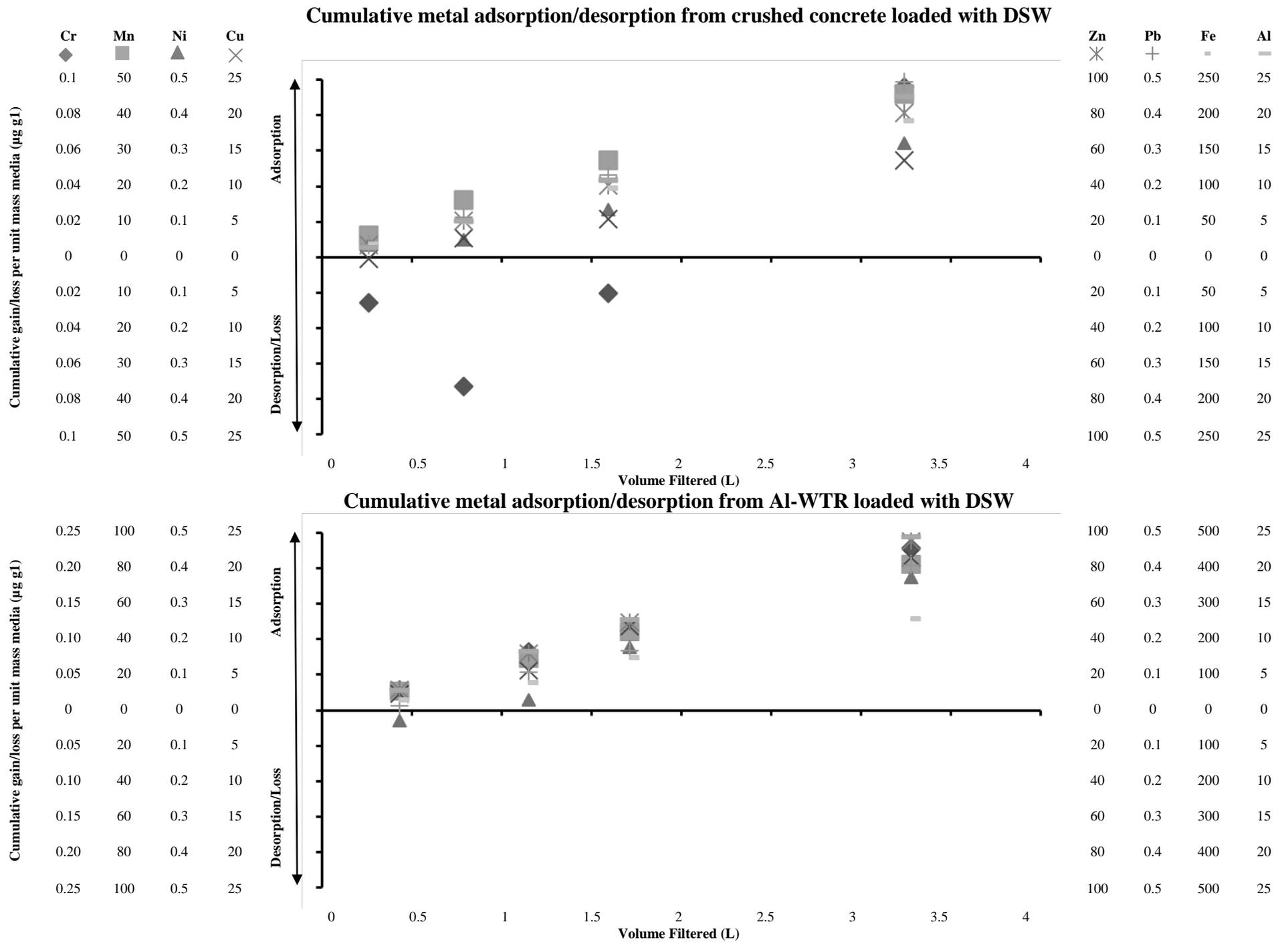
Figure 6.2 (b) Cumulative metal release/uptake by 0.4 m filter columns.
