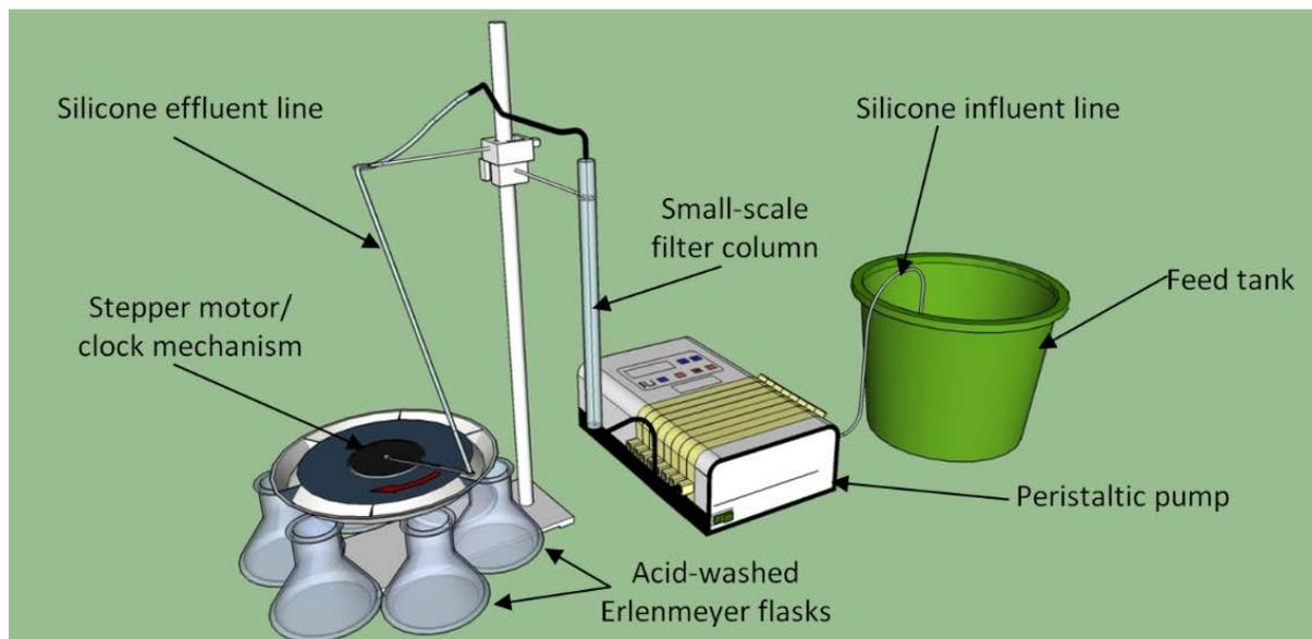
**Figure 2.2 Schematic of small-scale filter column experiment**
