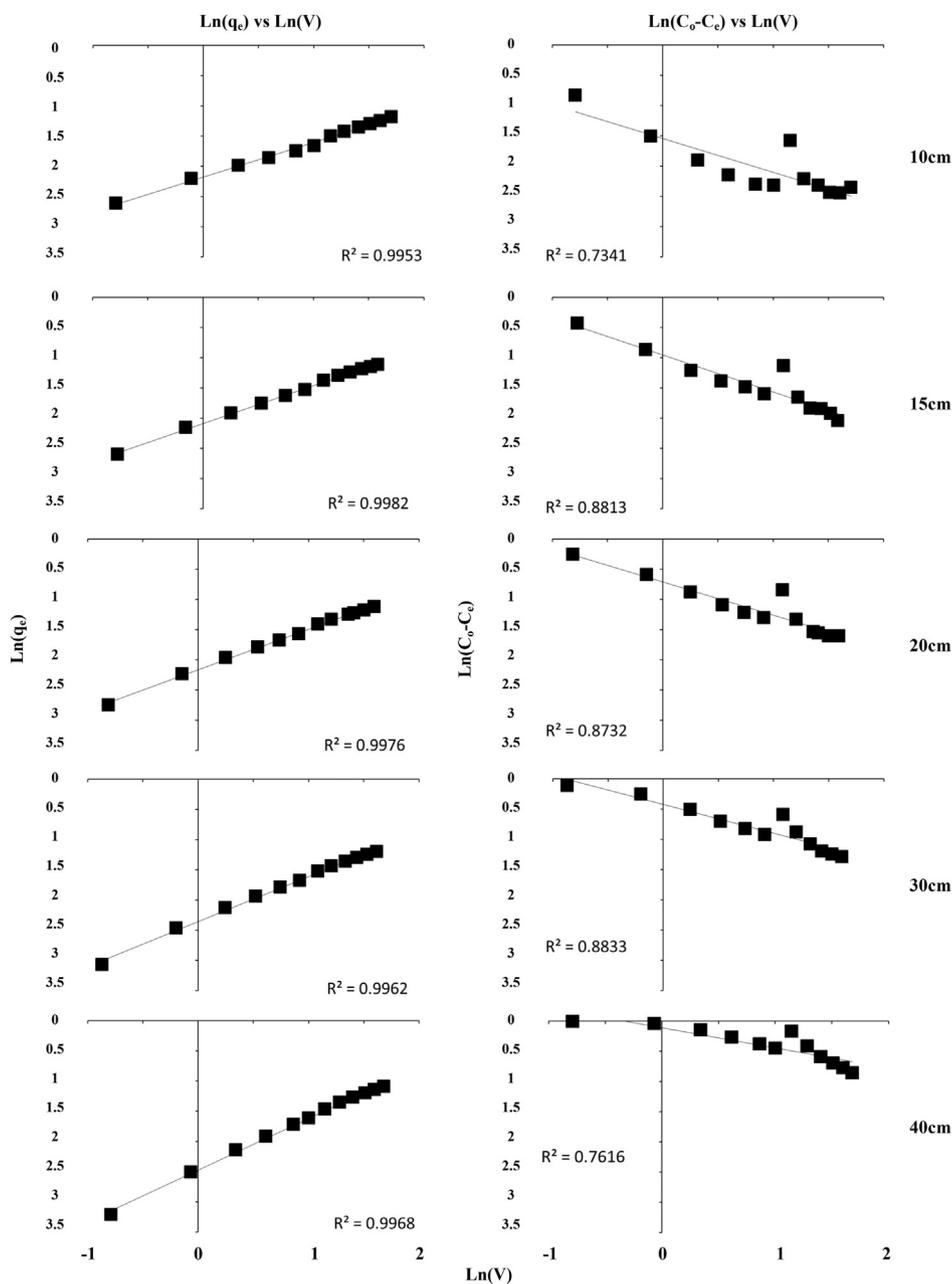
**Fig. 5.** Comparison of the linearity of plots of  $\text{Ln}(q_e)$  (left y-axis) vs.  $\text{Ln}(V)$  (x-axis), and  $\text{Ln}(C_o - C_e)$  (right y-axis) vs.  $\text{Ln}(V)$  (x-axis). These plots are used to determine model coefficients by analysis of filter saturation or filter effluent concentration respectively.
