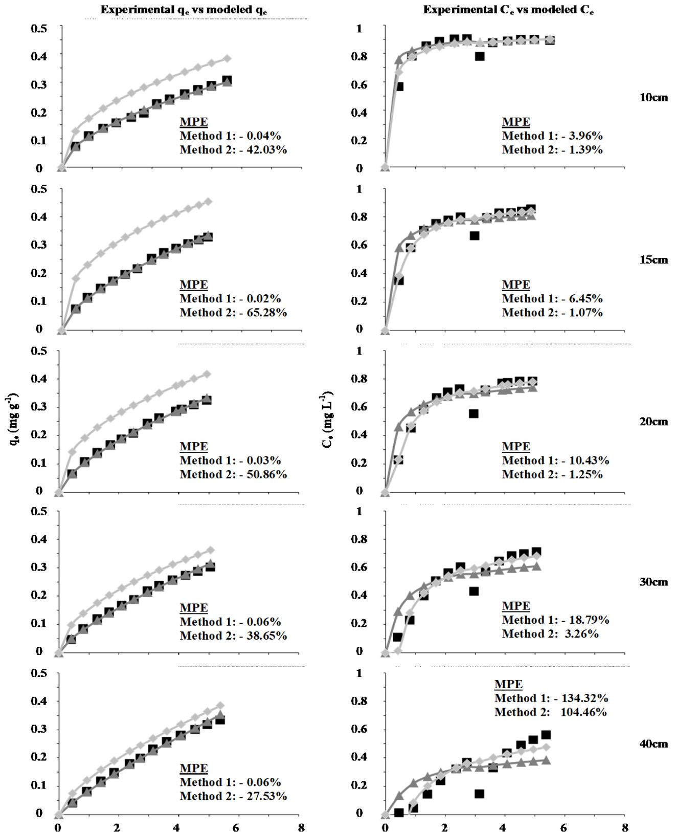
**Figure 4.6** Plots of  $q_e$  (left y-axis) and  $C_e$  (right y-axis) vs. filtered volume (x-axis), demonstrating the effect that the method of coefficient determination (ie analysis of filter saturation or analysis of filter effluent concentration) has on model accuracy.
