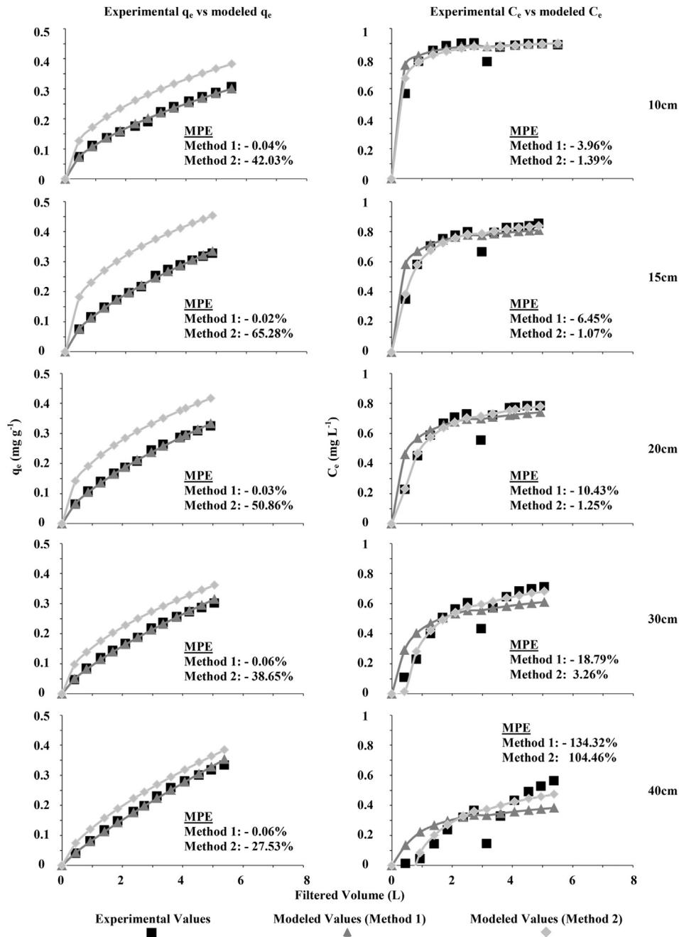
**Fig. 6.** Plots of  $q_e$  (left y-axis) and  $C_e$  (right y-axis) vs. filtered volume (x-axis), demonstrating the effect that the method of coefficient determination (ie analysis of filter saturation or analysis of filter effluent concentration) has on model accuracy.
