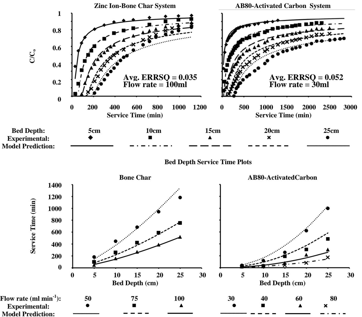
**Figure 5.6** (a) Equation 16 fit to an independent data set (Ko et al., 2002) of normalised effluent contaminant concentration (y-axis) vs. filter operating time (x-axis) for various filter-bed depths, and (b) plots of filter service-time (y-axis) vs. filter-bed depth (x-axis) compared to predictions made by Equation 17 using the same model coefficients
