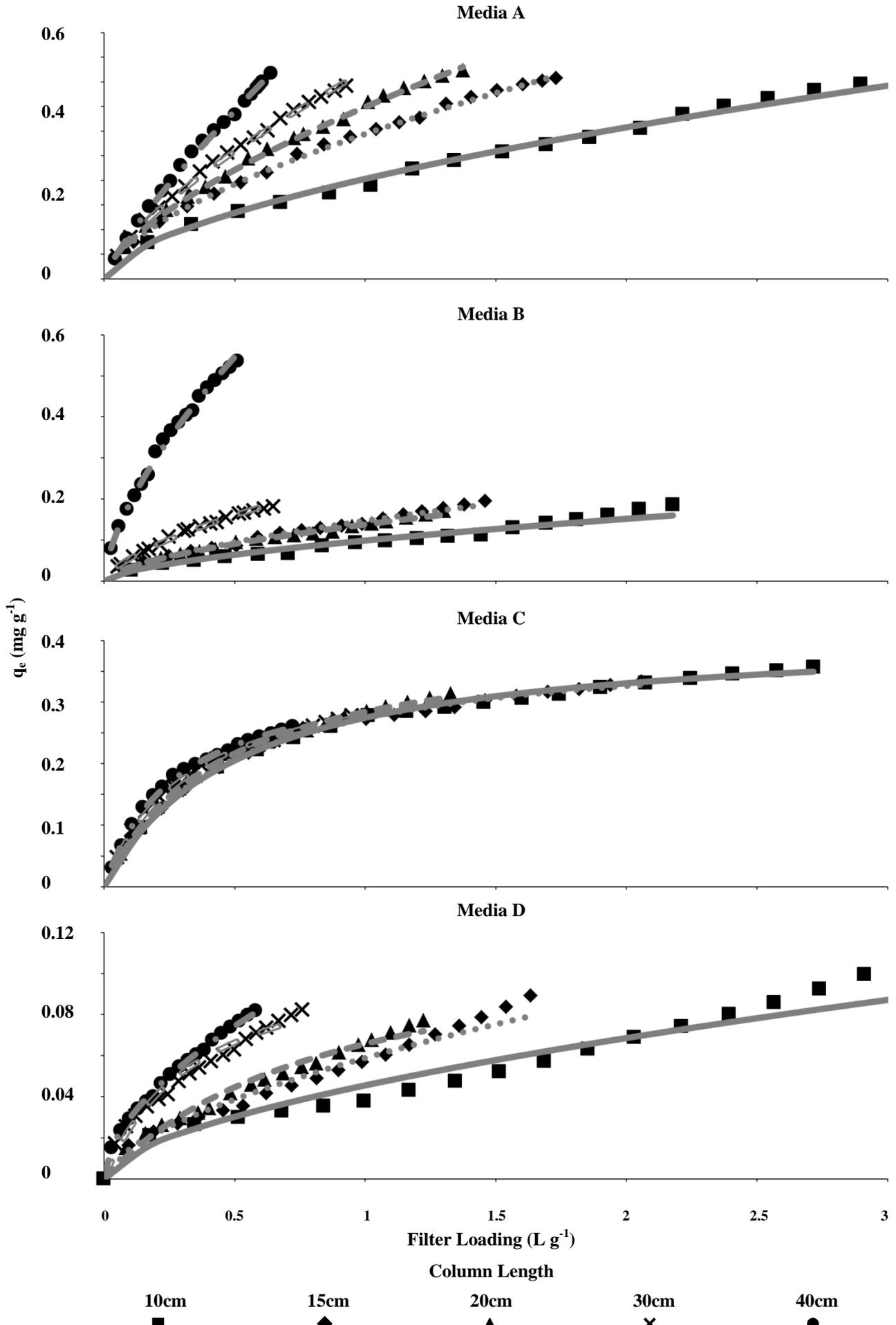
**Figure 4.1** Filter media P adsorption (y-axis) vs. filter loading (x-axis), showing observed progressions of media saturation and the goodness of model fit for each media and column length.
