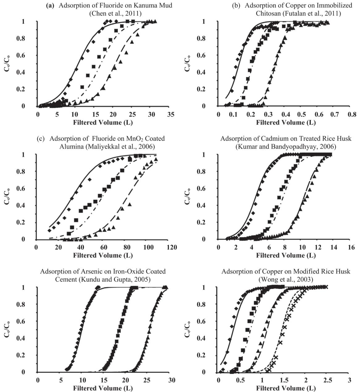
**Fig. 5.** Eqn (10) fit to independent data sets of normalised pore/effluent contaminant concentration (y-axis) vs. filter loading/operating time (x-axis) (Chen et al., 2011, Futalan et al., 2011, Maliyekkal et al., 2006, Kumar and Bandyopadhyay, 2006, Kundu and Gupta, 2005, Wong et al., 2003).
