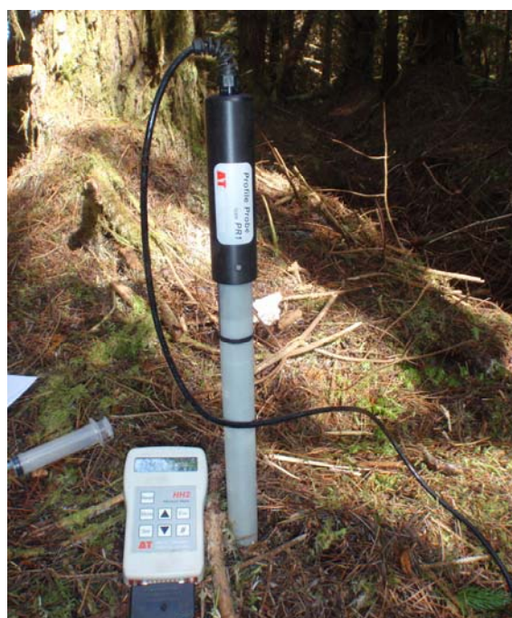
Figure 5.4 Soil volumetric water content equipment.
