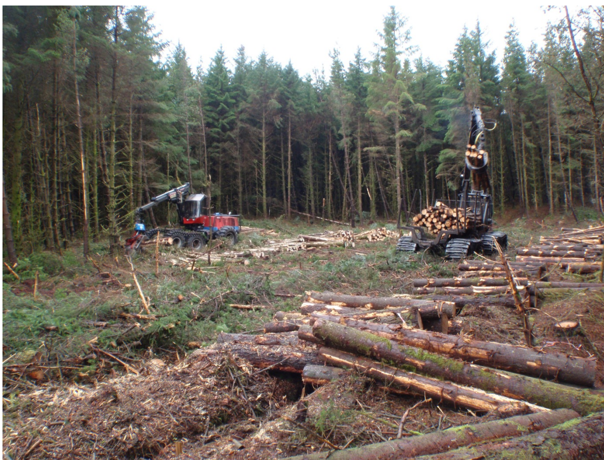
Figure 3.2 Valmet 921 harvester (on left) and Valmet 860 forwarder (on right).
