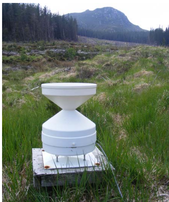
Figure 5.3 Rain gauge installed on site.
