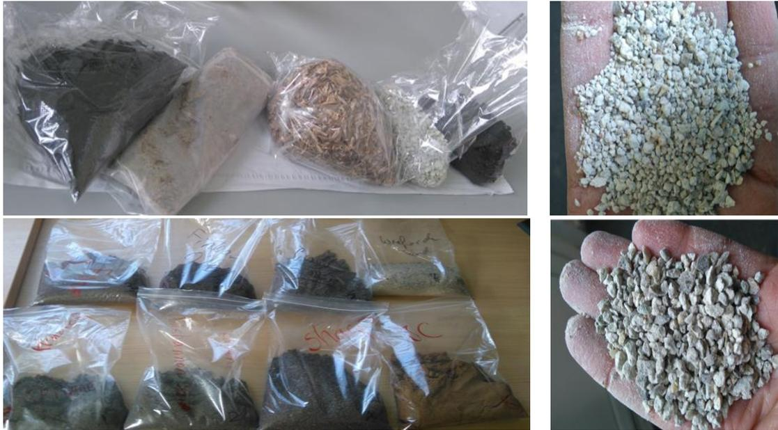
**Figure 5.1.** Some of the different waste materials used as in Table 5.1. Top left: Peat soil, sand, woodchip, zeolite, Puraflo<sup>TM</sup> (from left to right); Bottom left: Eight types of sand. Right column: Different grading of zeolite.
