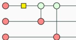
**Figure 4:** ZX-Diagram of GHZ State
